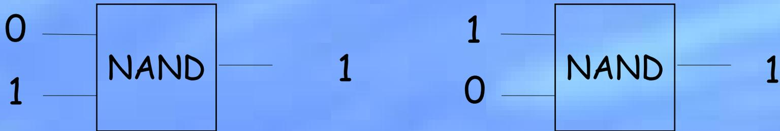
From the output of the NAND gate it is impossible to determine if the input was  $(0,1)$ ,  $(1,0)$ , or  $(0,0)$ .
